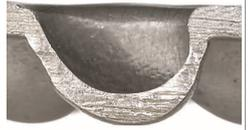
In the past, this problem was solved by using zinc - which had the necessary ductility - for the full shells (not the interchangeable ones).
